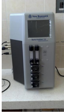
Fermentador/reactor New BrunswickScientific BIOFLO 115.
