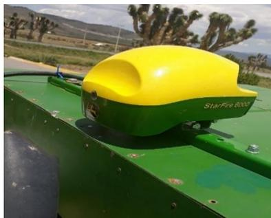
Figura 4. 8 Antena receptora GPS
