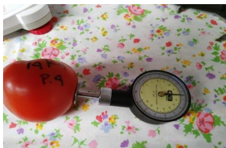
Figura 7 Penetrómetro manual FT Fruit Tester, Greenwich, Connecticut, EE. UU
