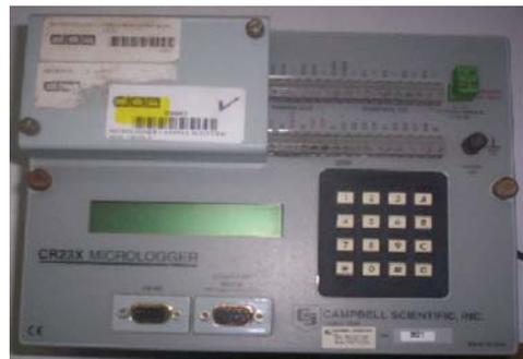
Figura 3.7 Micrologger Modelo 23 X de Campbell SCI.
