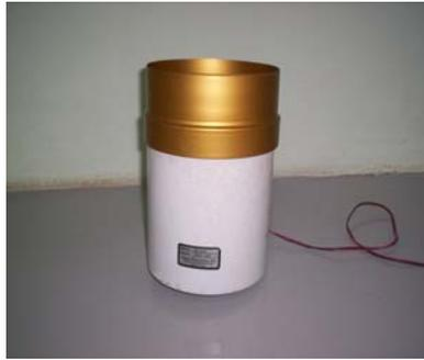
Figura 3.6 Pluviometro Texas Electronic, Modelo TR-5251
