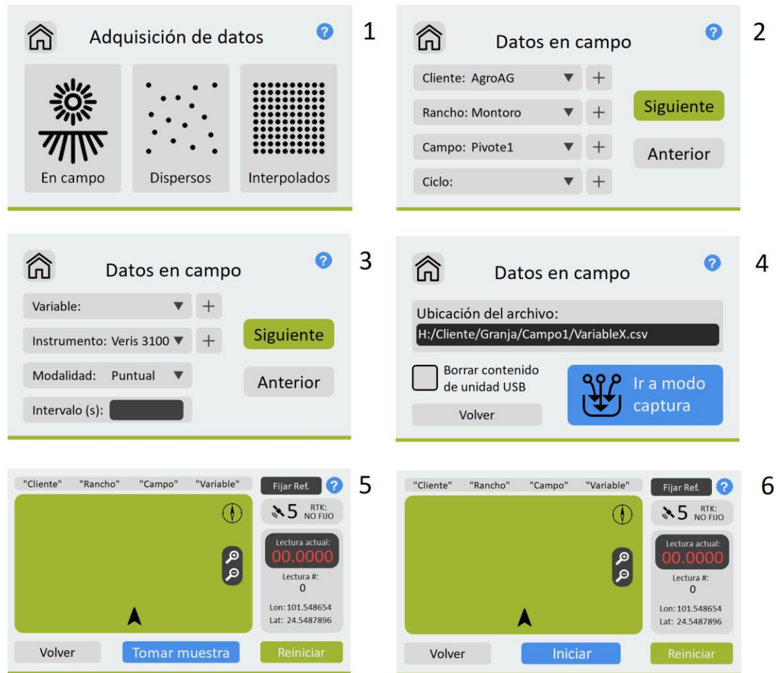
Figure 63. Data acquisition screens
