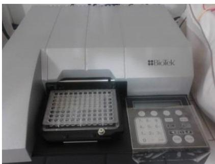
Figura 13. Lector de Microplaca (Bio- Tek Instruments).
